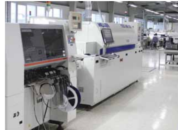
SMD production line
